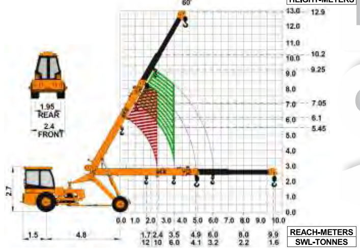
ACE 12 XW Model Crane fitted with 3 part slotted boom (12.90 mtrs. height)
