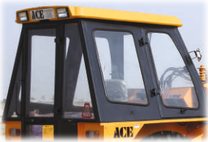
ROPS CABIN Wide view ROPS cabin for better visibility.
