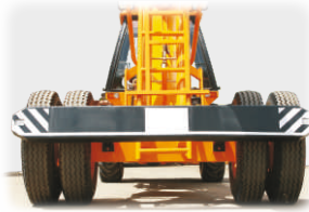
GROUND CLEARANCE High ground clearance of 400mm for easier rough terrain operation.
